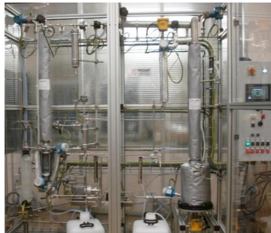
Figure 5: Absorption-regeneration micro-pilot unit at UMONS
