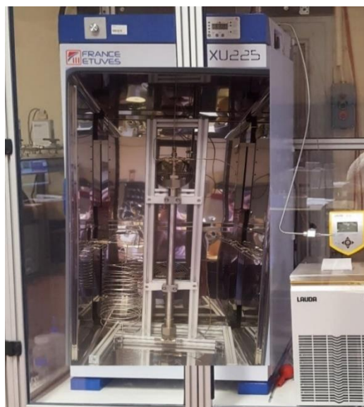
Figure 13: CO 2 catalytic conversion to methanol micro-pilot unit at UMONS
